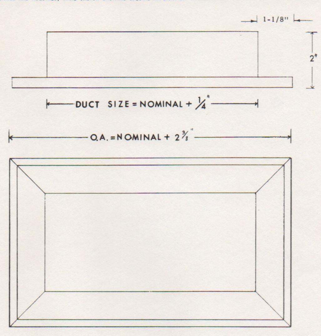
DESIGN: Aluminum frame having 3/8" larger dimensions than Register sizes. Its use allows two piece Register application, providing easy removal for cleaning.
